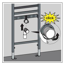
Mount the drain elbow.
