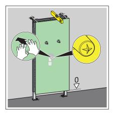
Corn the gypsum cardboard cladding panel at the plug using gentle pressure.
