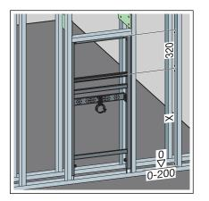
Set the installation height (X) of the element according to the ceramic manufacturer's instructions.
