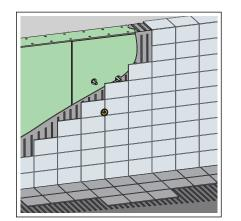
Clad the element with suitable gypsum cardboard cladding panels.
