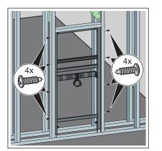
Attach the element to the support profiles using the screws supplied.
