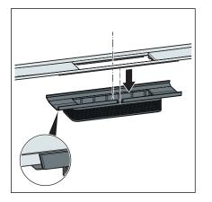
Insert the shower channel profile into the height adjustment piece as far as it will go.
