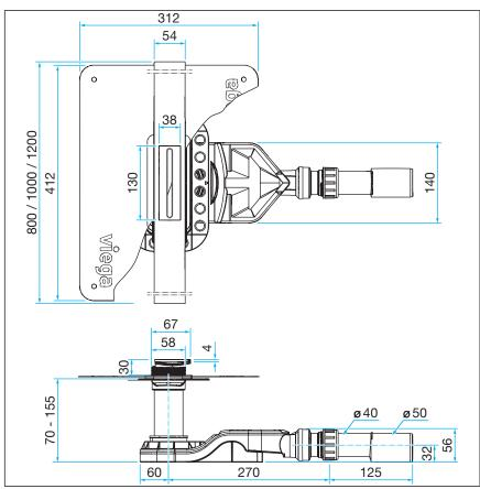
Fig. 3: Dimensions of base unit basic model
