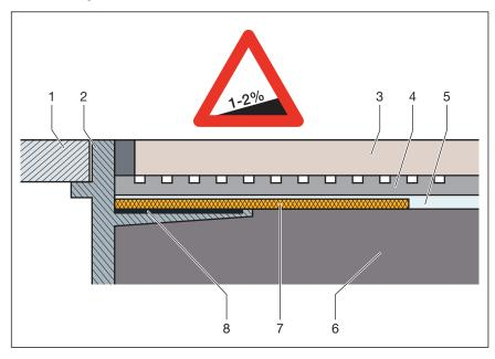
Fig. 2: Construction diagram of the bonded seal - min. screed incline 1–2 %
