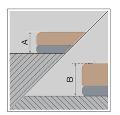
Due to the stepless shortening of the top, an installation height of at least A 12 mm to B 30 mm is possible for tiles and tile adhesive.
