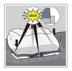
Push the sealing collar into the flange as far as it will go. All four fixing points must engage.
