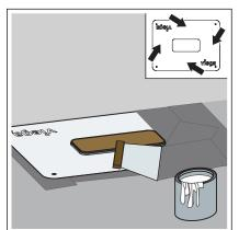
Once the first layer has dried, apply the second layer of the bonded sealing generously onto the sealing collar and screed.
