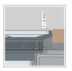
Lay the floor covering 1–2 mm higher than the shower channel profile.
