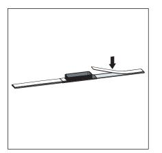
Stick the butyl tape centrally on the underside of the shower channel profile.
