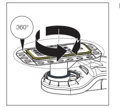
The flange can be rotated around 360°.
