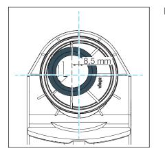
Turn the transition to eccentrically offset the drain by up to 8.5 mm.
