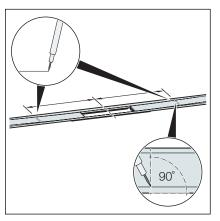
Determine the required dimension and mark at right angles.
