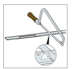
Using a handsaw, shorten the shower channel profile at right angles and deburr.
