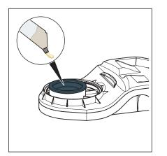
Apply a coat of lubricant for plastic pipes to the inside of the profile seal.
