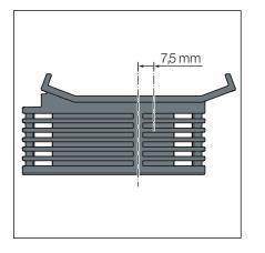
To allow the shower channel profile to be adapted to the tile pattern, the profile mount is eccentrically positioned by 7.5 mm.
