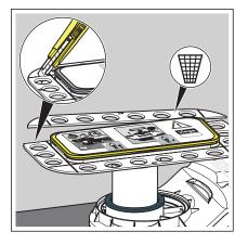
Cut the side of the reinforcement area on the wall with a blade. The flooring height (bonded sealing + adhesive + tiles) must not exceed 30 mm.
